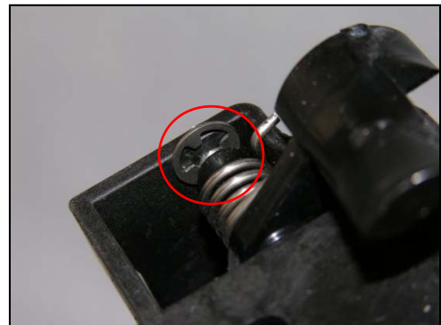
Figure 22: Tell-Tale Retaining Ring Not Seated
