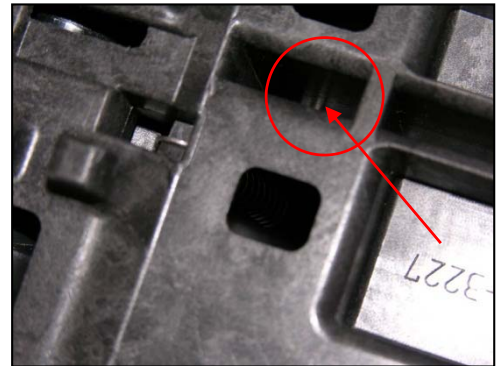
Figure 25: Return Spring Loops Shown Engaged
