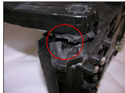
Figure 9: Operating Lever Shaft Kicker Broken
