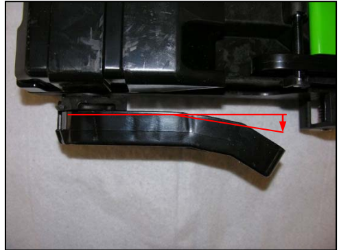
Figure 7: Operating Lever Handle Shown Bent
