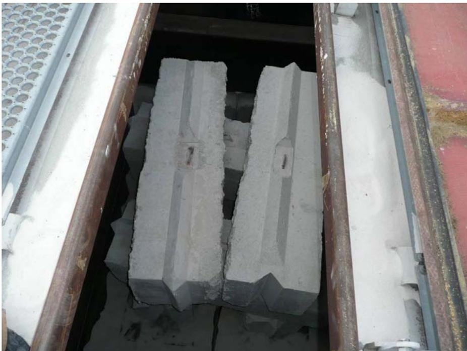
**PICTURE 5: LOADED CAR IMPACT TEST RESULT SHOWING 4 OZ. LEAKAGE AFTER 10 MINUTES**
