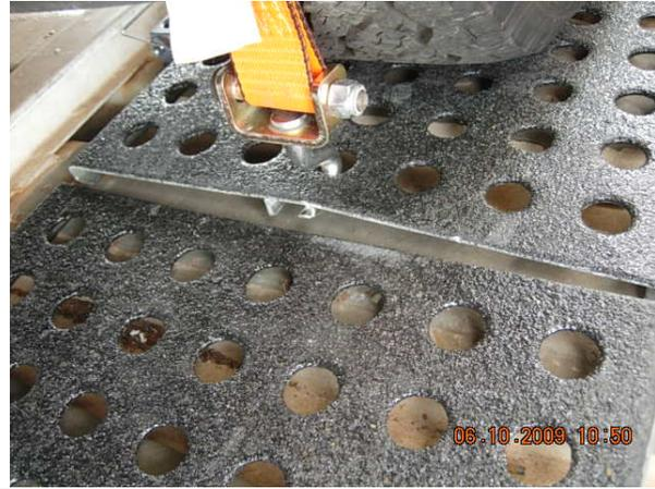
View of decking lifted by TrinityRail system.
